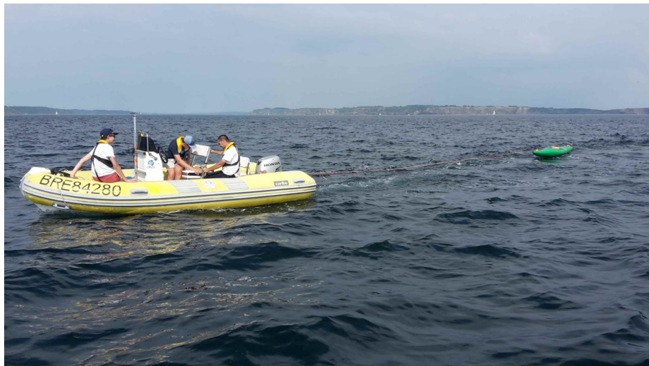
Figure 1.2: Picture of Boatbot towing a canoe towing a magnetometer.
