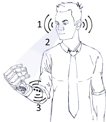
Fig. 4. Feedback system architecture. (1) Audio information (piezospeaker signals and sound of gearboxes); (2) Visual information (LED signals and movement of fingers); (3) Vibration of vibromotors.
