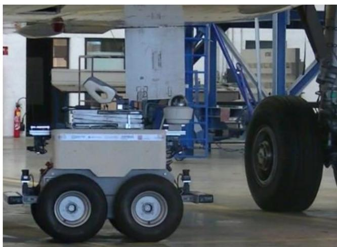
Fig. 1. Air-Cobot platform evolving under an A320 aircraft in a hangar of Air France Industries.
