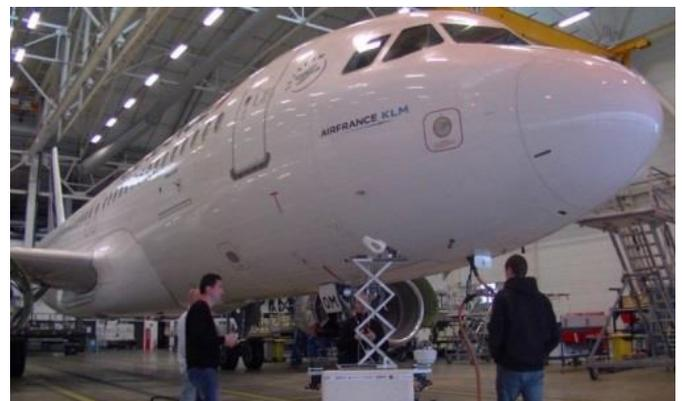
Fig. 14. Elevation of the scanner in order to perform a scan of A320 aircraft in a hangar of Air France Industries.
