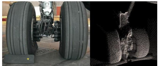
Fig. 11. At left, a picture from PTZ camera of a landing gear with a chock in front of the left tire. The task is the detection of the chock. At right, an example of laser data acquisition of a landing gear.
