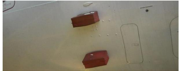
Fig. 12. Pitot probe protections are in place.
