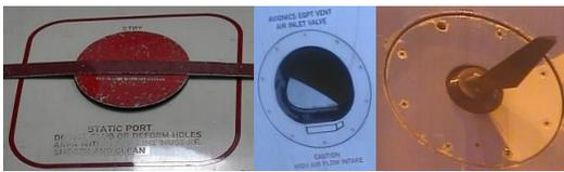
Fig. 8. Examples of items to inspect. From left to right, static port with its protection, open air inlet valve, AOA probe. Light conditions are very different.
