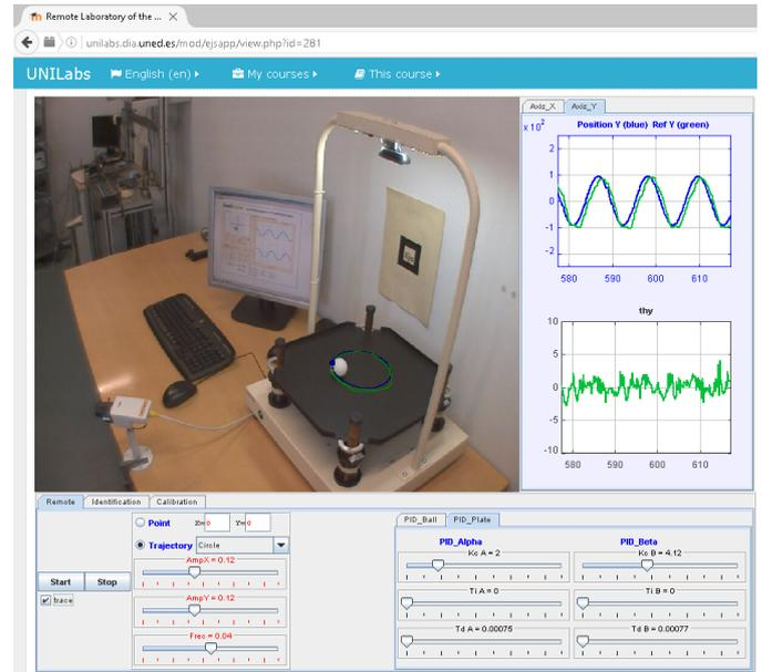
Fig. 9. Circular trajectory tracking experiment.
