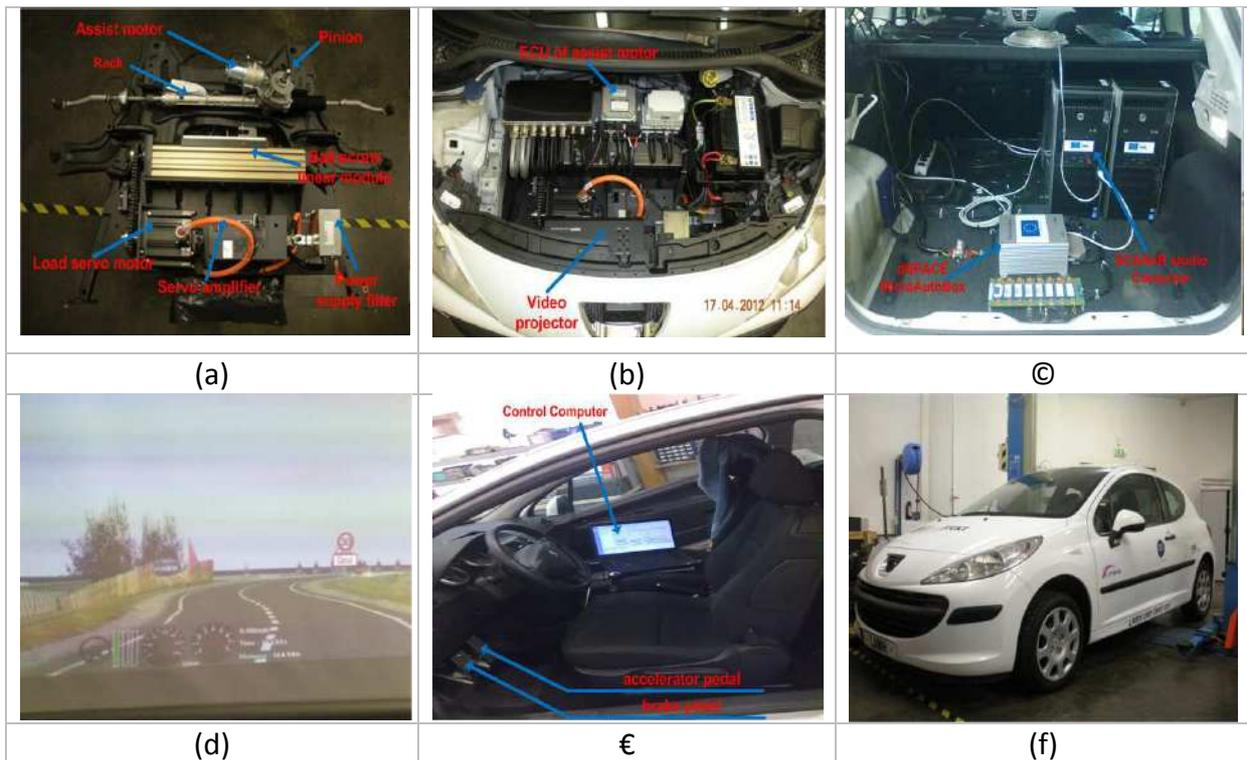
HIL simulator structure, (a) assist and load system, (b) assist and load system assembled in the engine compartment, (c) dSPACE MicroAutoBox and SCANer studio system, (d) Driving course and examples of the presentation screen, (e) driver's seat, (f) photography of the assembled HIL
