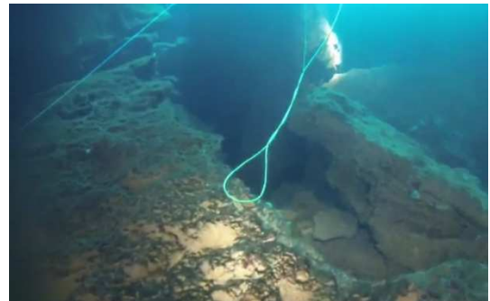
Fig. 5. The tether is making a loop. It is thus getting stuck around rocks. (Photo Credits : Mehdi Dighouth)
