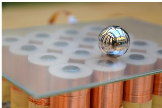
Fig. 1. The experimental platform consisting of a  $4 \times 4$  array of coils with an iron core. A steel ball is placed on a resistive touch foil for real-time position measurement.
