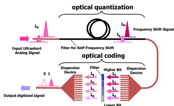
Fig.1. Schematic diagram of optical A/D conversion
