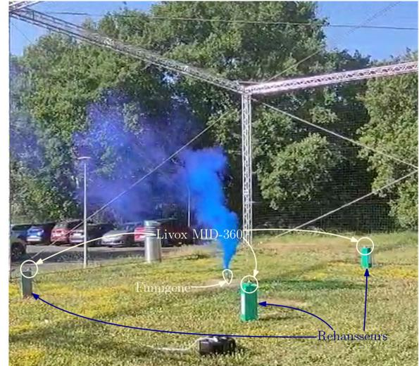
(b) *setup* for multi-LIDAR acquisition with 3 Livox MID-360 en extérieur
