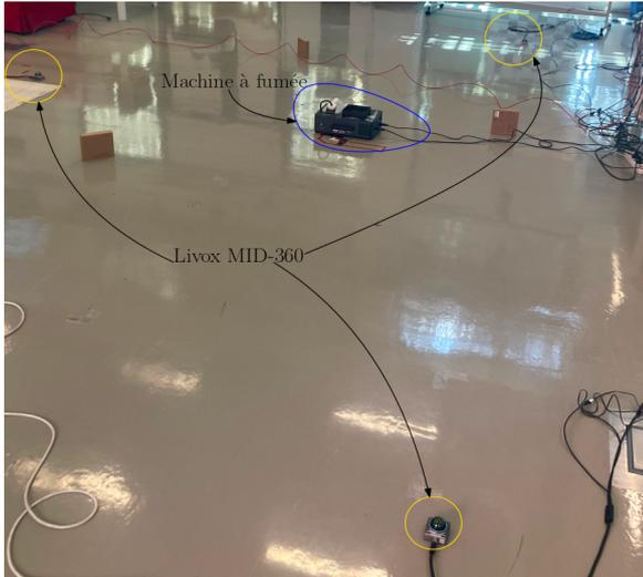
(a) *setup* for multi-LIDAR acquisition with 3 Livox MID-360 en intérieur
