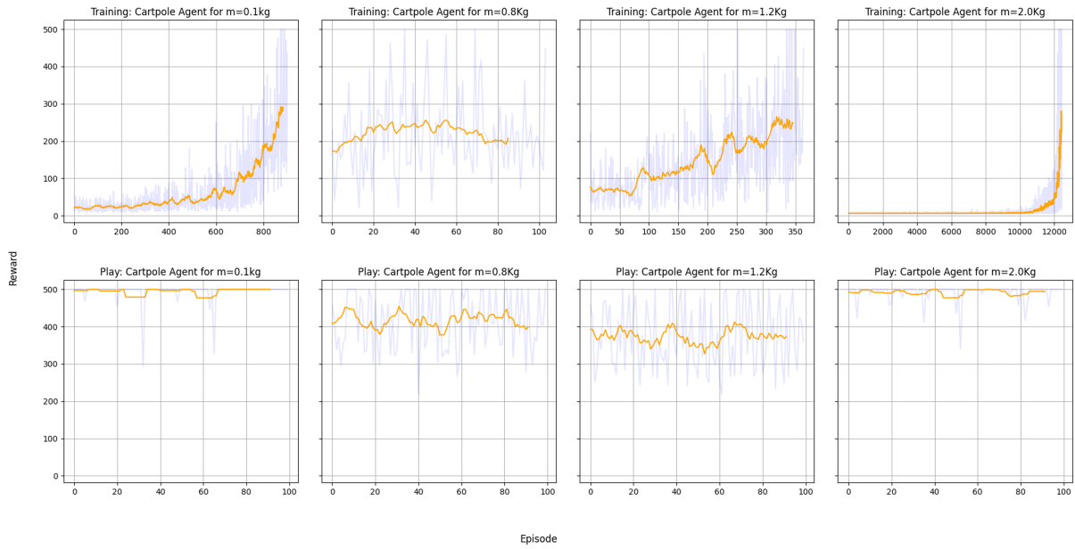
Figure 2.11: Sequential training with Wrapper-based knowledge transfer across Pole masses.
