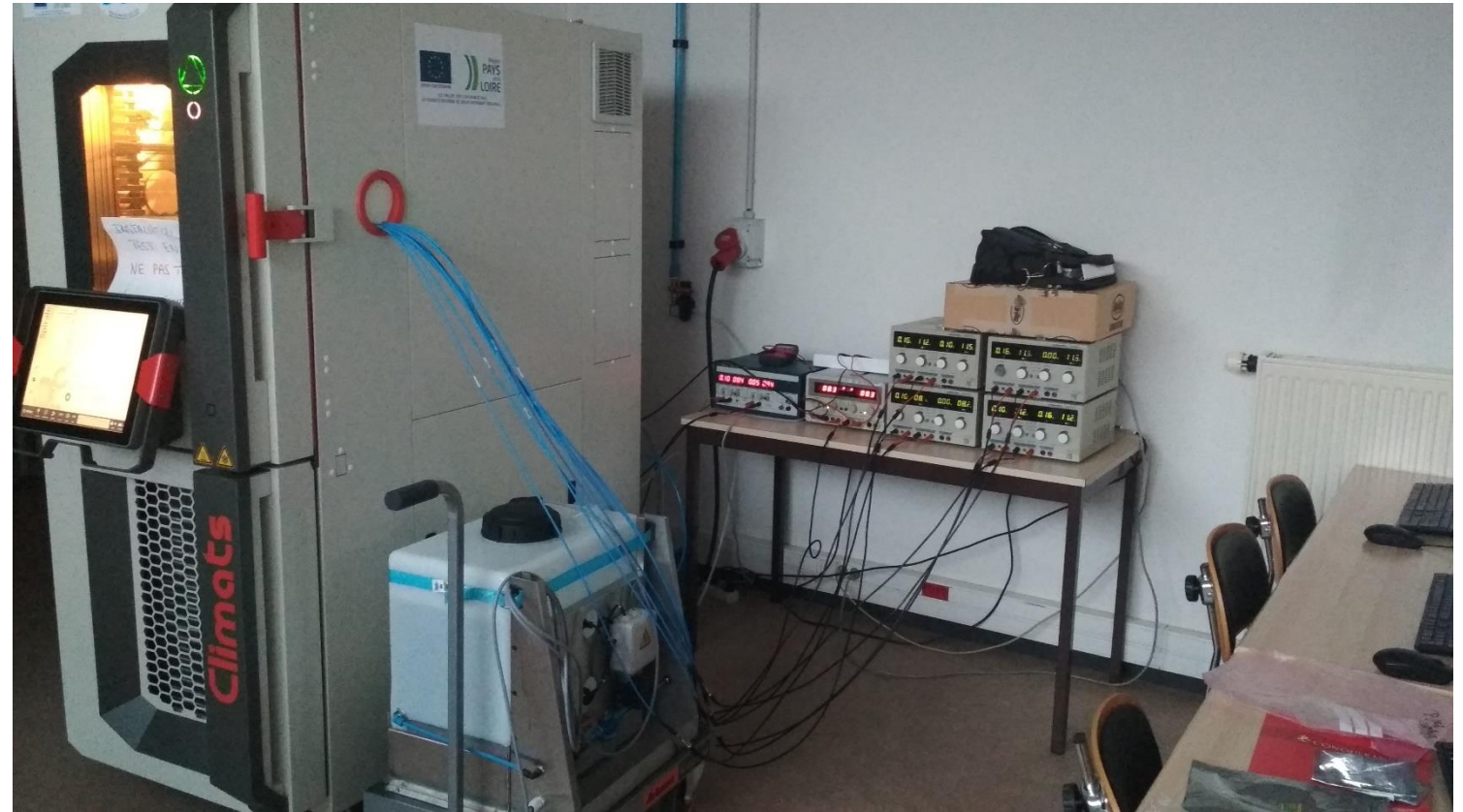
Climatic chamber for accelerated ageing test
